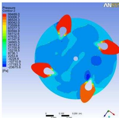
**Figure 6.** Pressure distribution in a plane at Y-axis
