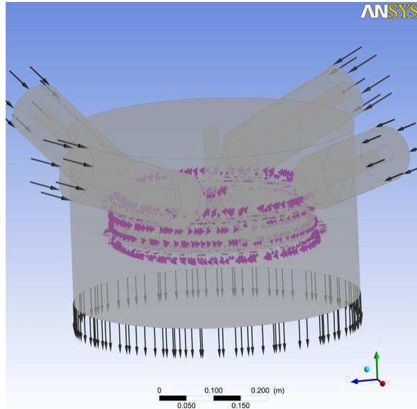
**Figure 5** Boundary condition of whole setting
