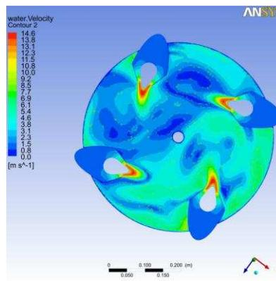
**Figure 7.** Velocity distribution in a plane at Y-axis
