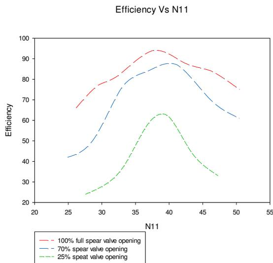
**Figure 11.** Speed factor vs efficiency graph
