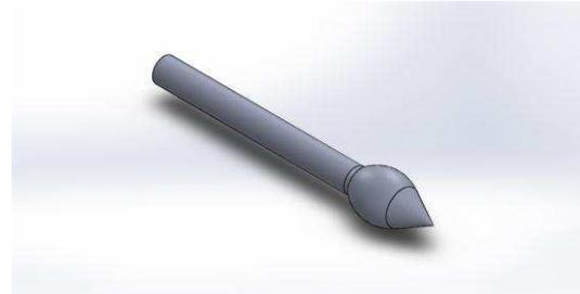
**Figure 2.** Spear valve design
