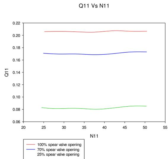
**Figure 12.** Speed factor vs Discharge factor
