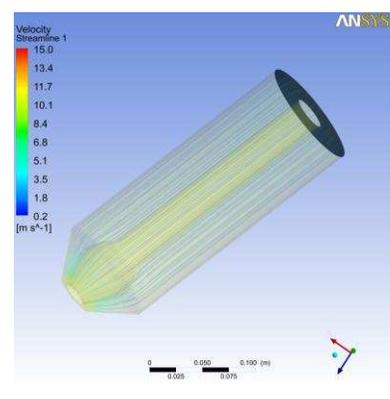
**Figure 8.** Streamline flow in a nozzle
