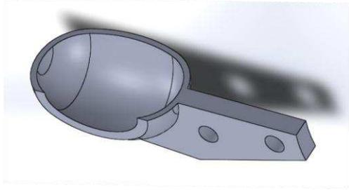
**Figure 1.** The basic bucket stem design for clamped or bolted fixing
