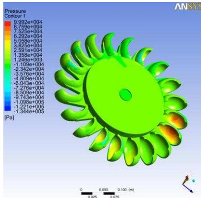
**Figure 9.** Pressure distribution in runner
